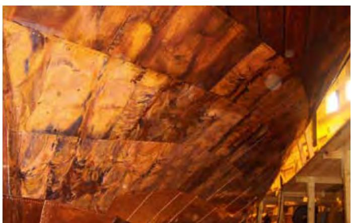
The copper has been annealed to follow the contour of the hull.
